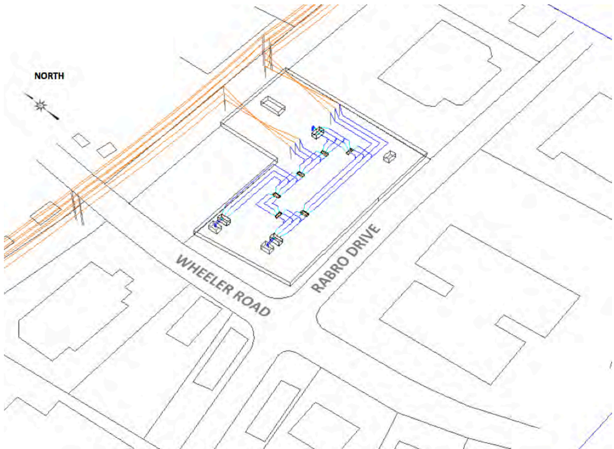
Figure 4. Overview of the three-dimensional SUBCALC model used to calculate magnetic-field profiles in the vicinity of the proposed Kings Highway Substation for the average and peak loading cases.
