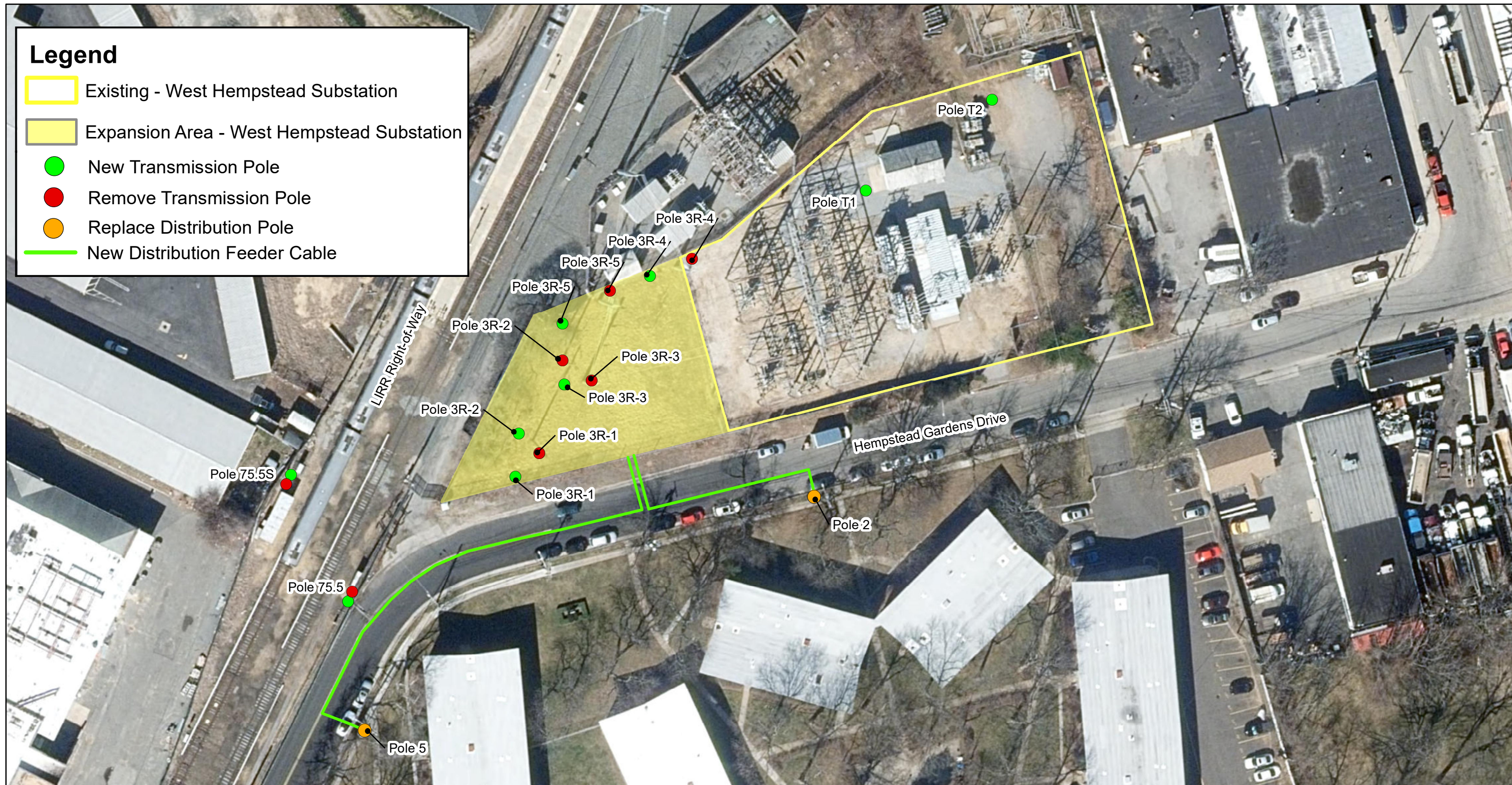
FIGURE 2 WEST HEMPSTEAD (3R) INSTALL FOUR 69/13kV 33MVA TRANSFORMERS AND ASSOCIATED WORK TOWN OF HEMPSTEAD, NEW YORK SITE PLAN
