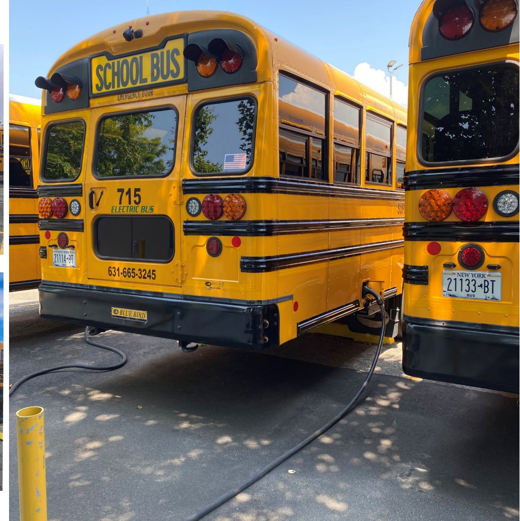
Bluebird Vision Generation - 2 EV Buses With 156 KW Battery with a range of 80-120 Miles.
