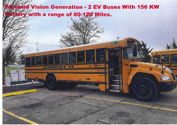
Bluebird Vision Generation 1 EV Buses Hooked up to Level 2 Chargers
