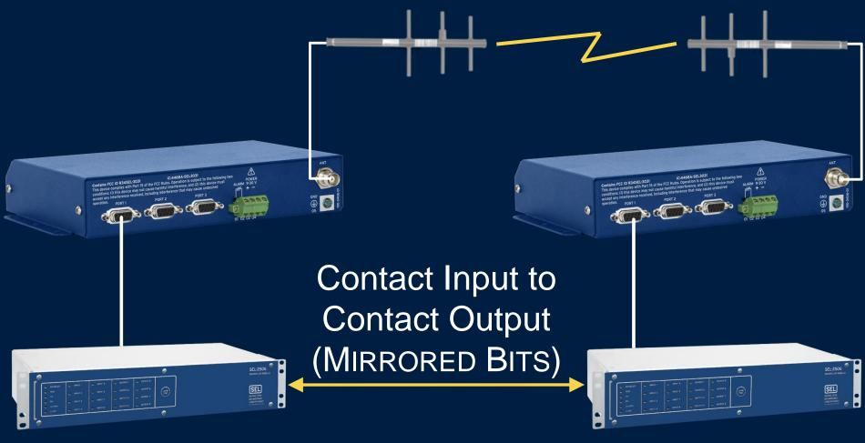
Unencrypted = 8.8 ms Encrypted = 13.4 ms
