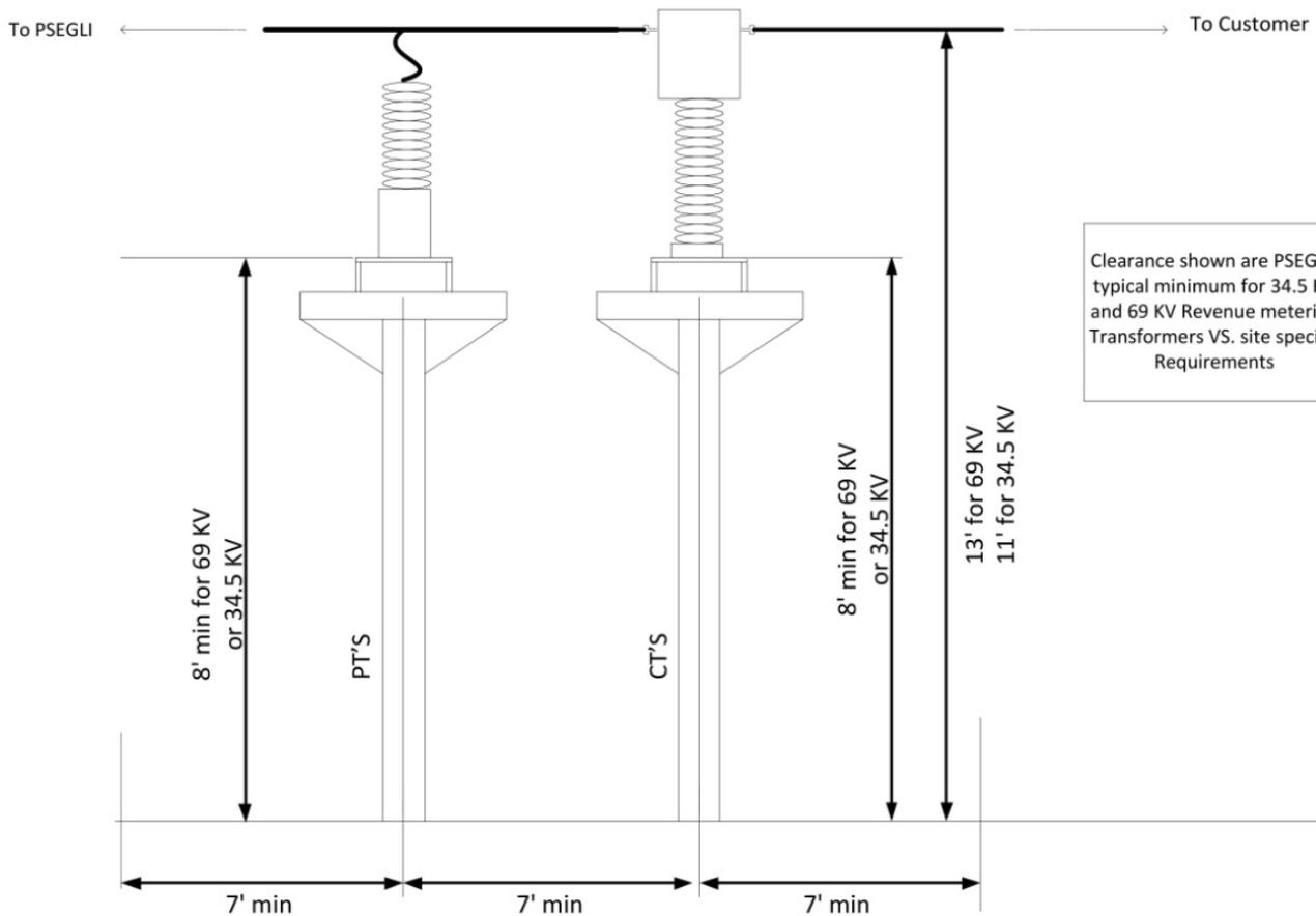
Clearance shown are PSEG-LI typical minimum for 34.5 KV and 69 KV Revenue metering Transformers VS. site specific Requirements
